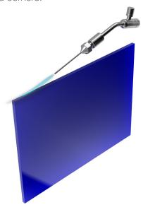
The torch should be held at a slight angle and the flame drawn along the edge of the sheet. If the first pass does not produce a completely polished edge, the piece can be allowed to cool and then a second pass performed.
