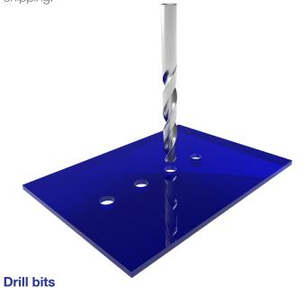
Drill bits specifically designed for plastics will always work best. However, conventional HSS twist drills can be used if reground to give a tip angle of 60-90° and a flat cutting edge with a rake angle of 0-4°.
