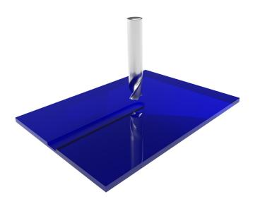
The tendency of acrylics to craze can inhibit their ability to be machined at high speeds, especially during cutter entry, as router bits do not have a centering point similar to drills due to the requirement for flat bottom cutting. Excessive spindle speeds may also melt the acrylic or result in a poor finish.
